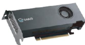
SupremeRAID™ SR-1010 is the world's fastest GPU-based RAID controller for PCIe Gen 3, 4, and 5 servers -- designed to deliver superior NVMe/NVMeoF, SAS, and SATA performance while increasing read/write in all flash array and HPC applications.
